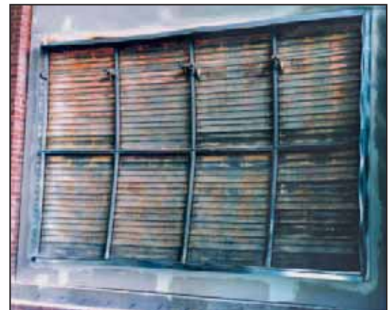
Photograph of actual UL 555 fire test conducted successfully at Underwriters Laboratories Inc., Northbrook Illinois.
