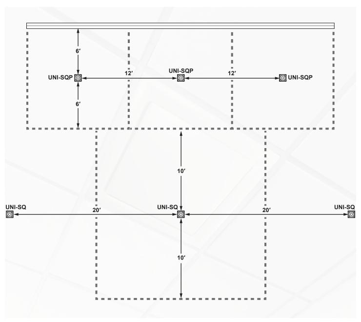
By utilizing a combination of **UNI2-SQ** and **UNI2-SQP** diffusers, the designer will have a similar looking diffuser in both interior and perimeter zones while minimizing drafts due to jet collisions and also meeting perimeter heating requirements.
