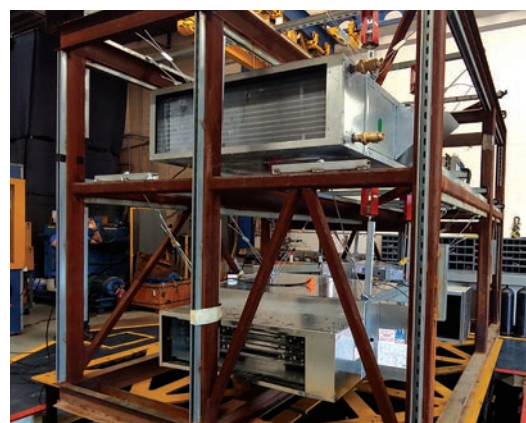
Fan Powered Terminal Units Shake Table Test
