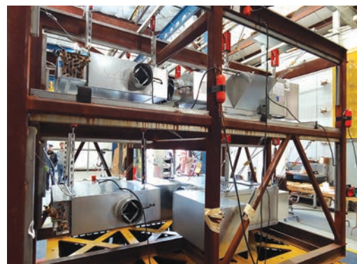
Fan Powered Terminal Units Shake Table Test
