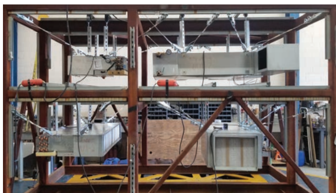
Horizontal Fan Coil Units Shake Table Test
