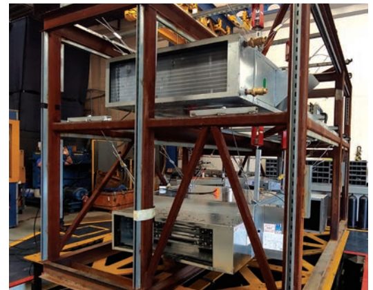
Fan Powered Terminal Units Shake Table Test
