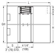
MODEL 0130G: TYPE CR ROUND DUCT CONNECTION ON ONE END GH = DIA. + 2" (51)
