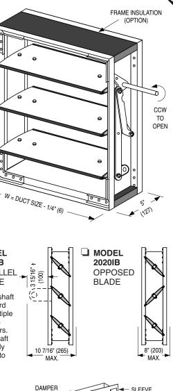
SLEEVE FRAME OR DUCT LOCK-ON OUTBOARD DRIVE SUPPORT SHAFT BEARING BRACKET OUTBOARD SUPPORT BEARING
