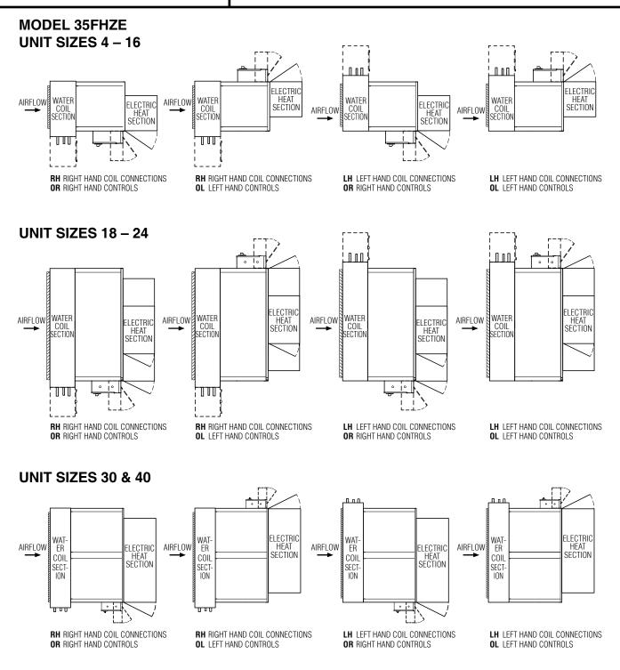
NOTE: Optional Outside Air Inlet (OAI) available on unit configurations where controls and coil connections are on the same side.
