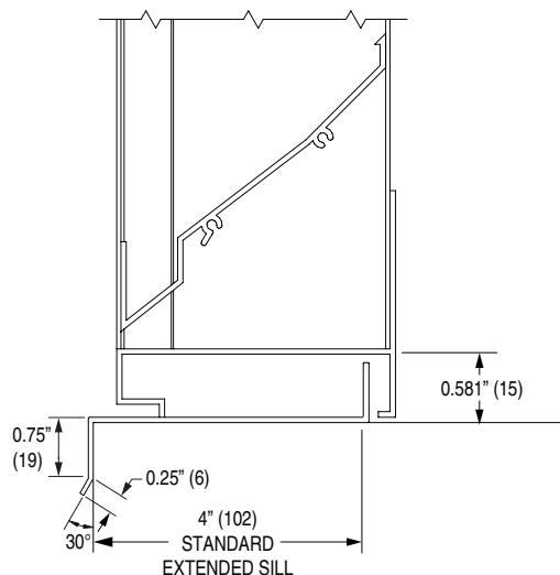
**PASI** Sill Pan (Extended Sill with End Dams)
