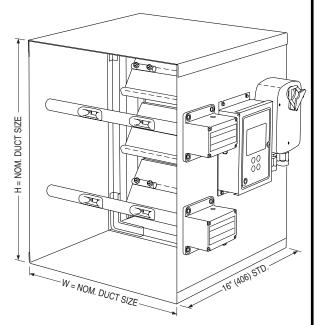
Performance Data - Air Leakage (Damper Closed) 3.5 cfm/ft² @ 1" w.g. (64 cmh/m² @ .25 kPa) 7 cfm/ft² @ 4" w.g. (128 cmh/m² @ 1 kPa)
