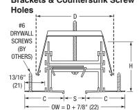
☐ Type CCCA Concealed Tapered Side Frame with Concealed Mounting Brackets & **Countersunk Screw Holes**
