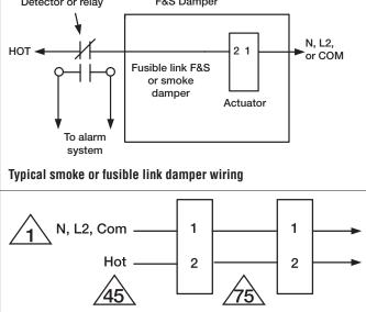
Parallel Actuator Wiring
