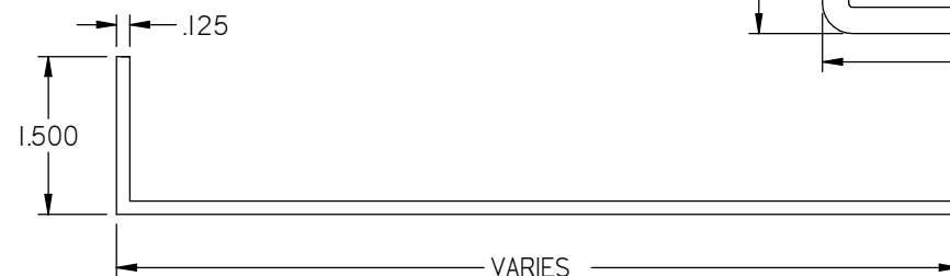
16 SLEEVE FORMED ALUM. 5052-H32 ALUMINUM
