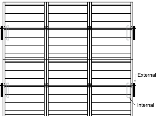
Detail 32S 3 Sections Wide 2 Sections Tall 4 Actuators
