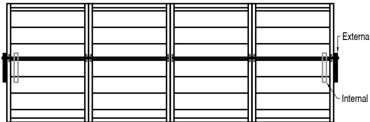
Detail 41S 4 Sections Wide 2 Actuators, 1 per 2 sections
