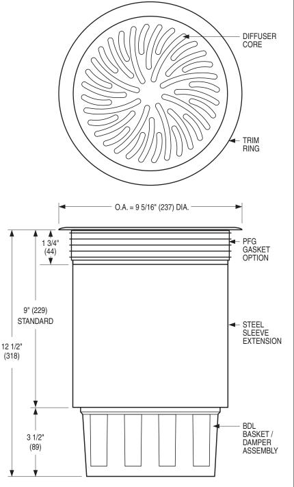
**NOTE:** Hole opening requirement in floor for installation = 8.375" (213) diameter. Tolerance +/- 0.03125" (0.8)
