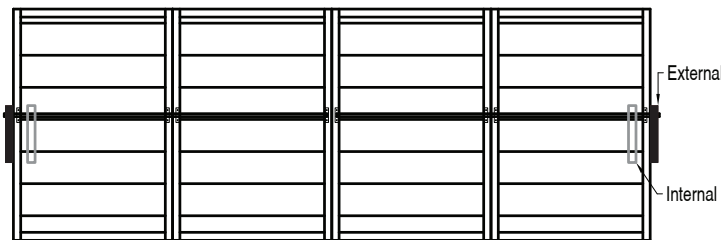
Detail 41S 4 Sections Wide 2 Actuators, 1 per 2 sections
