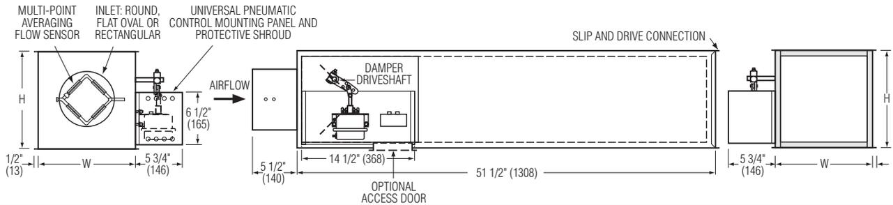
**AT Discharge Sound Attenuator (loose)**
