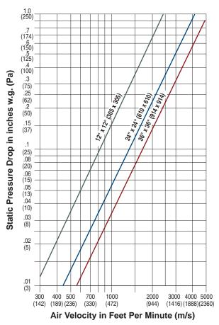
Pressure drop tested per AMCA Standard 500-D, Figure 5.3. Data corrected to standard air density of 0.075 lbs/ft.<sup>3</sup>.
