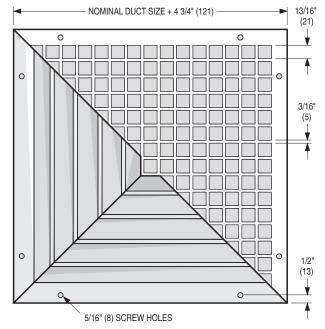
**Model SG-6500** is most often used in minimum security areas such as lobbies and foyers where constant supervision is required. This ceiling diffuser assembly combines the high performance **Model Series 6500 Pattern Diffuser** with a heavy gauge steel lattice grille mounted on the diffuser face. Also optionally available in aluminum construction as **Model SG-6200**.
