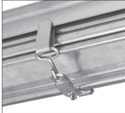
All Nailor curtain type fire dampers are equipped as standard with a UL Listed fusible link that will melt, or 'fuse', when it is subjected to its rated melting temperature, allowing the damper to close. 165°F (74°C) fusible link is provided as standard. 212°F (100°C) is also available (See Closure Temperature Options).
