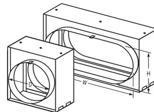
Blades and frame out of the airstream; used mainly for transitioning to round or oval duct. Provides optimum pressure drop characteristics with blades and frame out of airstream.
