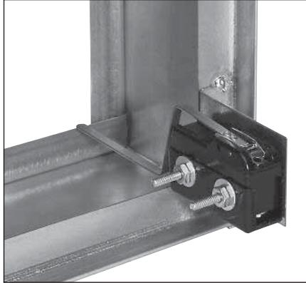
Option Code MS provides any Nailor fire damper with a factory mounted micro switch suitable for use in low voltage (24V) applications. Activated when the damper blades are closed, the switch can be used for status indication of damper when wired into a control panel or can be utilized to shut a fan off upon closure of damper. UL and CSA approved single pole, double throw switch is rated up to 15 amps. and can be wired up as normally closed or normally open, depending upon application.
