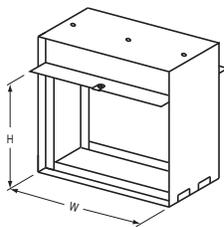
Blades out of the airstream; With blades out of airstream, provides better free area and resulting pressure drop characteristics than Type 'A', especially on smaller size dampers.
