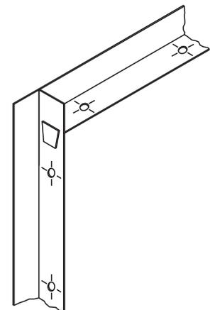
**Style 1:** 1 1/2" x 1 1/2" x 20 ga. (38 x 38 x 1.0) Four sides are connected together with rivets in three corners. Standard for the majority of applications with the following limitations:
