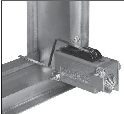
Option Code MSE, microswitch with enclosure, provides a factory mounted micro switch similar to Option MS, except the MSE with its safety enclosure is suitable for use in line voltage (120V) applications. Similarly, the MSE can be used for status indication or fan shut down and also can be wired for normally closed or normally open applications. Enclosure is tapped with 1/2 inch NPS threads for conduit connection and is also provided with an internal earthing (ground) screw.
