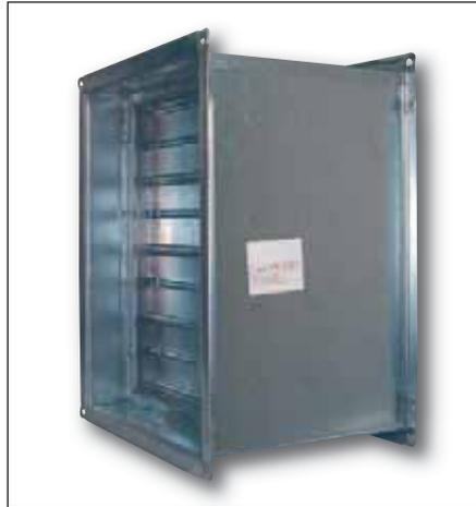
**TDF** (by Engle) and **TDC** (by Lockformer) proprietary flange systems are approved as breakaway connections for connecting a factory sleeved (22 or 20 gauge) Type A or B curtain type fire damper to ductwork. They may be used in place of the approved slip joints shown in standard installation instructions.
