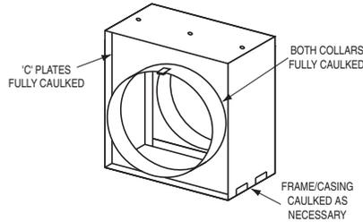
Sealed for use in medium and high pressure applications up to 6" w.g. (1.5 kPa), Type C fire dampers with HP option are externally caulked to minimize leakage through casing and collars.
