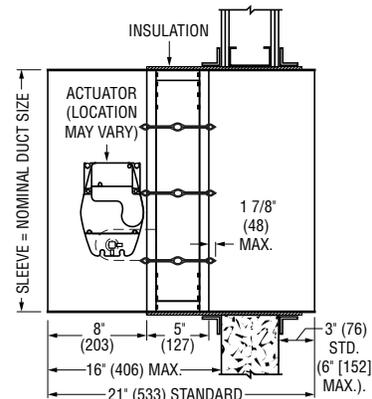
**NOTE:** STANDARD SLEEVE/DAMPER (FOR 4" [102] WALL) PROVIDES 1" (25) OFFSET FROM WALL FACE TO EDGE OF DAMPER FRAME. FOR THICKER WALLS OR TO OFFSET DAMPER FARTHER FROM WALL FACE (MAX. 8" [203]) LENGTHEN SLEEVE ACCORDINGLY.
