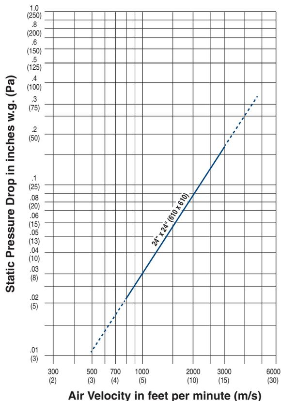
Pressure drop tested per AMCA Standard 500-D, Figure 5.2.
