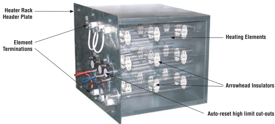
Figure 5: Typical element rack for a series Fan Powered Terminal Unit
