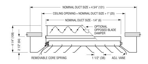
Minimum duct size: 6 x 6 (152 x 152). Maximum duct size: 36 x 36 (914 x 914) or 36 x 24 ( 914 x 610) with O.B.D. Available in 3" (76) increments only.
