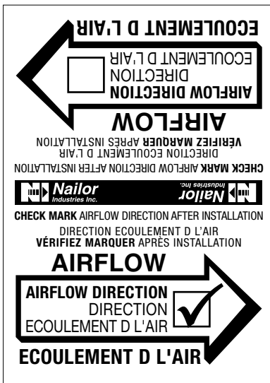
Figure 5: Example of check marked label showing the Correct Direction of Airflow (From Left to Right in this case).
