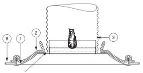
FOLD BACK NECK FLAPS OF THERMAL BLANKET. SLIP FLEXIBLE DUCT OVER THE NECK OF THE DIFFUSER.
