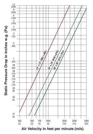
Pressure drop tested per AMCA Standard 500-D, Figure 5.3. Data corrected to standard air density of 0.075 lbs/ft.³.
