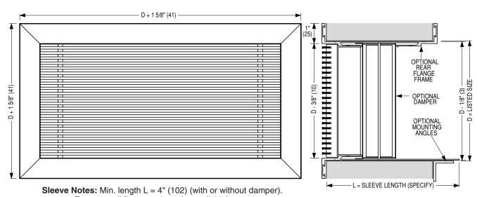
For rear wall flange option -L = wall thickness. For mounting angle option -L = wall thickness + 2" (51).
