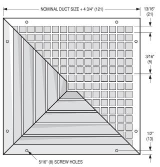
**Model SG-6500** is most often used in minimum security areas such as lobbies and foyers where constant supervision is required. This ceiling diffuser assembly combines the high performance **Model Series 6500 Pattern Diffuser** with a heavy gauge steel lattice grille mounted on the diffuser face. Also optionally available in aluminum construction as **Model SG-6200**.
