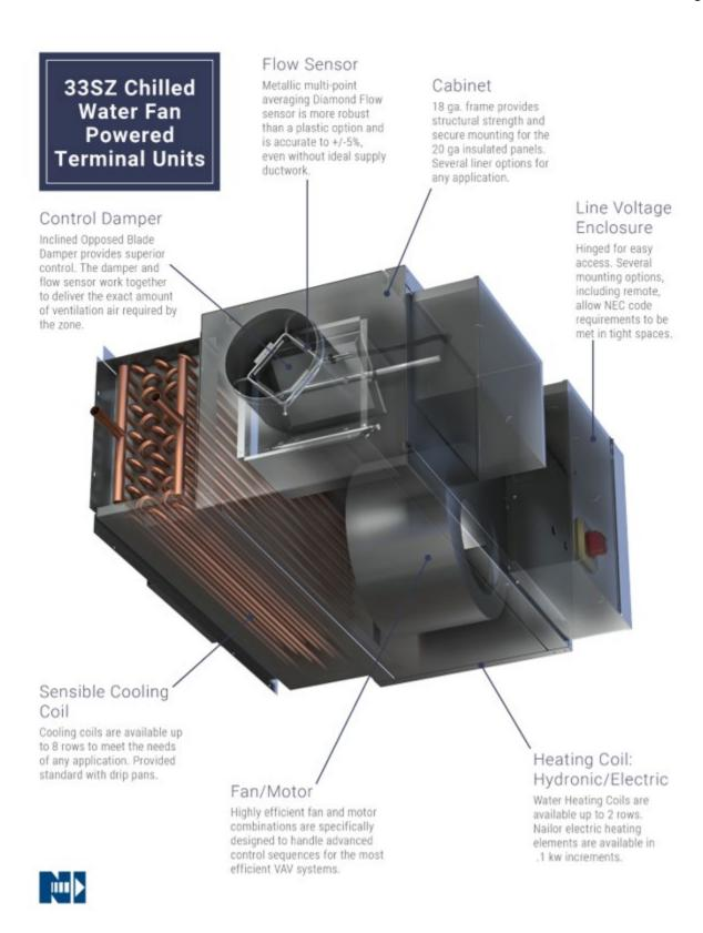
The fan in the terminal unit is responsible for delivering the ventilation air to the space. Because the fan is in series with the airflow, the DOAS system fan is only required to deliver the ventilation air to the terminal unit.
