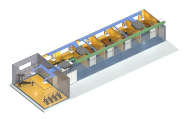
The latent load is handled by the dry air from the DOAS air handling unit. Also, the building exhaust ensures the room air is replaced throughout the day.
