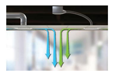
While this design satisfies the code, the two airflows do not mix in the space. This little-known phenomenon causes stratification of the air in the room, allowing some areas to receive more ventilation air than others. Nailor has performed detailed testing to prove this at Energistics Laboratory in Houston, TX. Regardless of air volume and temperature differences between the recirculated and ventilation air, airflows stay independent in the room.
