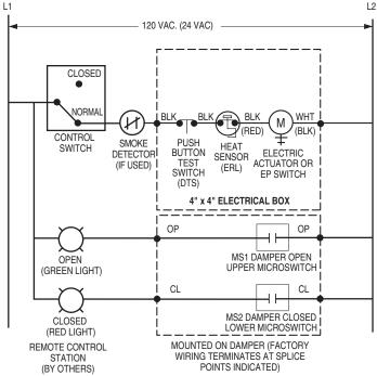
Figure 2. DTS/ERL with MLS-300 Belimo (actuator aux. switches)
