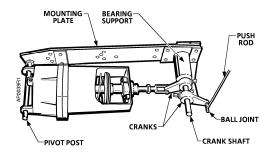
Figure 9. Extended Shaft Remote Mounting Assembly.
