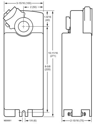
Fig. 1. Dimensional drawing of actuator in in. (mm).
