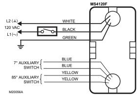
Fig. 8. Typical 120 Vac wiring (MS Series).
