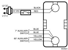
Fig. 3. Typical 24 Vac wiring.
