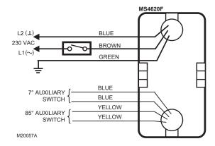
Fig. 9. Typical 230 Vac wiring (MS Series).
