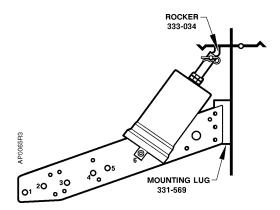
Figure 8. No. 4 Actuator Frame Mounting, Normally Open Damper.
