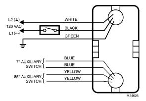
Fig. 4. Typical 120 Vac wiring.
