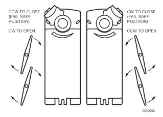
Fig. 2. Spring Return DCA mounting orientation.
