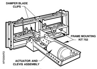
Figure 5. Two-section Damper.
