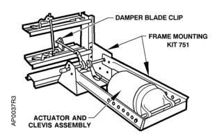
Figure 3. One-section Damper.
