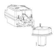
Figure 4. GJD Actuator and EFL.
