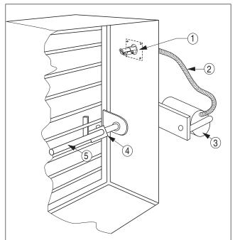
Typical Combination Fire/Smoke Damper Detail with UL Listed Pneumatic Actuator Description:
