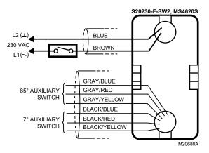
Fig. 11. Typical 230 Vac wiring (S20 Series).
