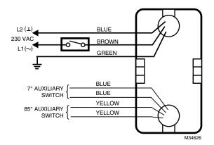
Fig. 5. Typical 230 Vac wiring.
