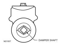
Fig. 3. Proper mounting to square damper shaft.
