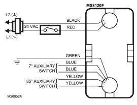
Fig. 7. Typical 24 Vac wiring (MS Series).
