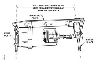
Figure 4. Perpendicular Mounting.
