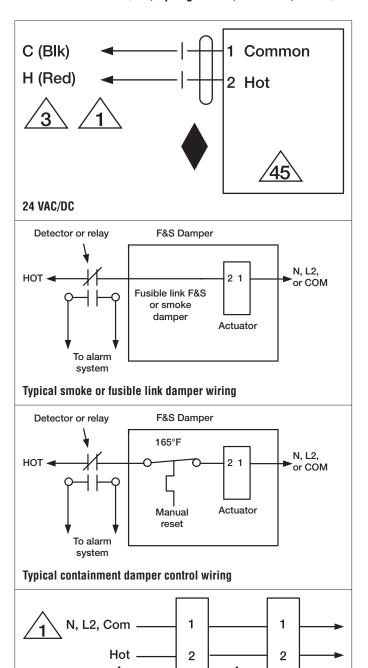
**Parallel Actuator Wiring**
