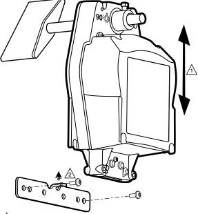
/1\ ENSURE THAT MOUNTING ASSEMBLY PREVENTS ACTUATOR ROTATION AND ALLOWS ACTUATOR TO FLOAT ALONG INDICATED AXIS. WHEN TOO TIGHT, THE RESULTING BINDING CAN DAMAGE THE ACTUATOR OR REDUCE TORQUE OUTPUT.
