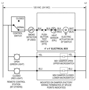
Figure 3. DTS/ERL with MLS-300 Nailor or Honeywell (actuator aux. switches) Position Indicator Package
