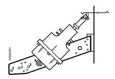
Figure 8. No. 6 Actuator Frame Mounting, Normally Open Damper.
