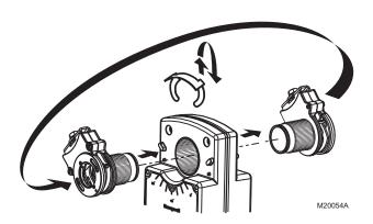
Fig. 4. Mounting shaft coupling to actuator opposite side.
