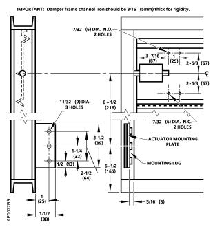
Figure 6. Frame Mounting Dimensions. Dimensions in Inches (Millimeters).
