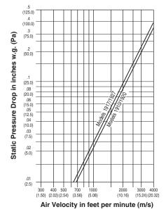
Tested per AMCA Standard 500-D using test set-up Figure 5.3, ductwork upstream and downstream.
