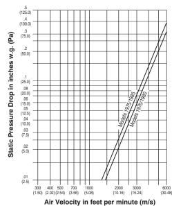
Tested per AMCA Standard 500-D using test set-up Figure 5.3, ductwork upstream and downstream.
